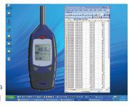
spreadsheet applications. Data stored within the CEL-246 can also be accessed since these meters act like a memory stick, allowing transfer of data to spreadsheet applications.
